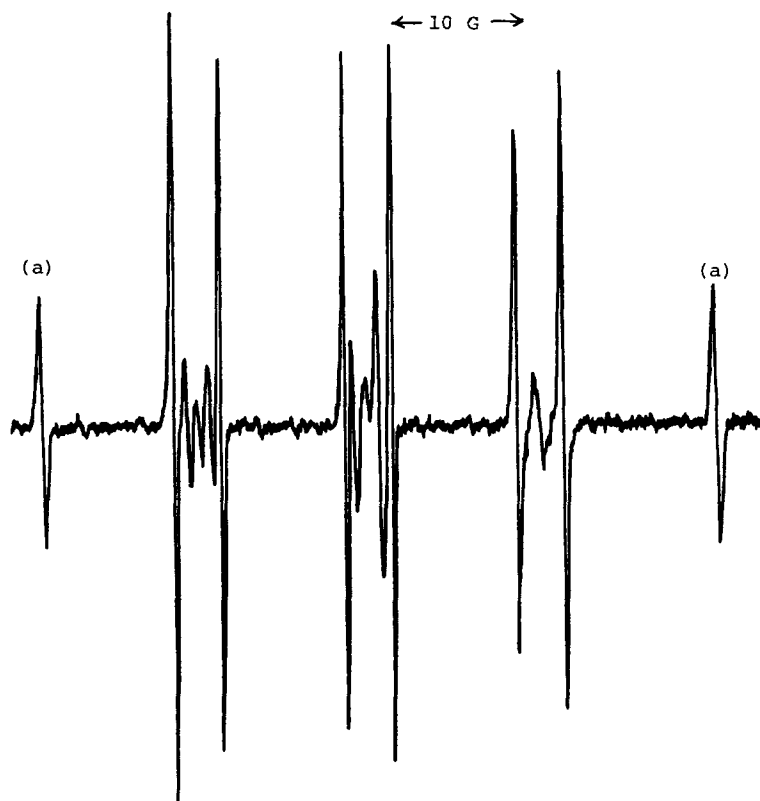
FIG. 9. ESR spectrum of the reaction system ethyl acetoacetate/di-tert-butyl peroxalate (DBPOX)/BNO after being reacted for 1 h at room temperature. (a): N -tert-Butoxy-tert-butylaminyl oxide, [DBPOX] = 4.3 \times 10^{-2} , [BNO] = 2 \times 10^{-2} mol/L.
